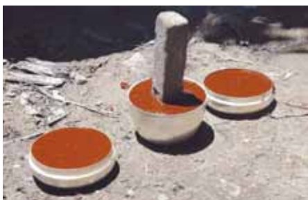
Figure 133: Silver articles with lac support ready for engraving.
