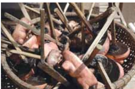
Figure 134: Silver articles with lac support ready for engraving.
