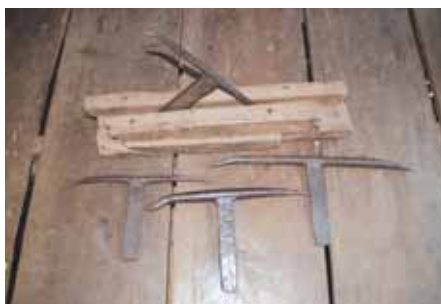
Figure 119: Anvil placing for work.
