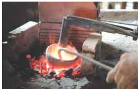
Figure 110: With help of fire above from blow pipe.
