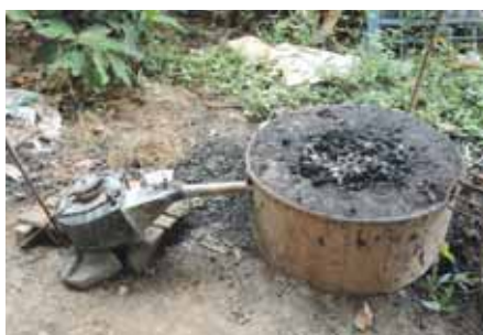
Figure 104: Motor using in car air conditioner is attached to forge to replace traditional bellows.
