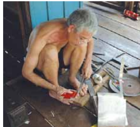
Figure 116: Silversmith cut silver into size by using a paper model.
