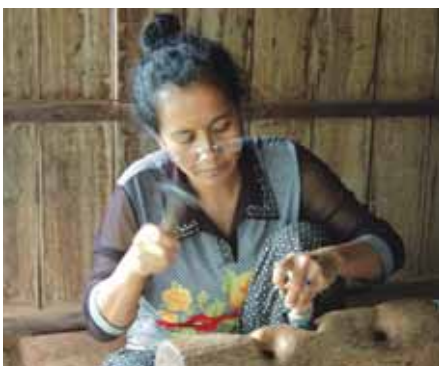
Figure 135: A wooden stick is attached and inserted into any hole of a wooden bar when engraving.
